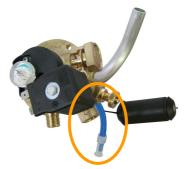
The withdrawal pipe is the pipe that allows the withdrawal of lpg from the bottom of the tank. The withdrawal is made because of pressure difference between the tank and outside. The pipe can be plastic or metallic, dependiong on multivalve version.
