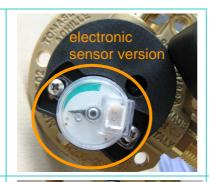
The magnetic group guides magnetically the external level indicator that could be a mechanical pointer or an electronic sensor; in case of electronic version, the sensor is connexed by a wire to the switch inside the car, and indicates the quantity of lpg inside the tank
