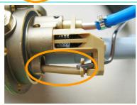
The magnetic group is made by a plastic part that holds a magnet; the movement of the float rod, due to different lpg levels inside the tank, create a rotation of the magnet holder that is used to move the external level indicator.
