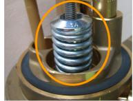
The pressure relief valve is a valve with a retaining spring that allows the relief of the lpg in vapour phase from the tank, in case of overpressure (27 bar), to avoid the explosion of the tank. In toroidal multivalves the safety valve is inside a plastic or aluminium pie, that has the function to let release only lpg in vapour phase.
