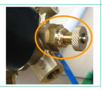
Device for the manual closing of the gas at the outlet, in case of mainteinance of the system.
