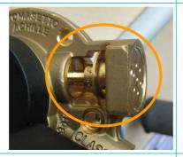
Device with a thermofuse element that in case of fire melts at predetermined temperature of  $120 \, \text{C}$ , this allows the opening of a big hole in the valve body, for the fast release of the gas from the tank, in order to avoid the explosion of the tank.
